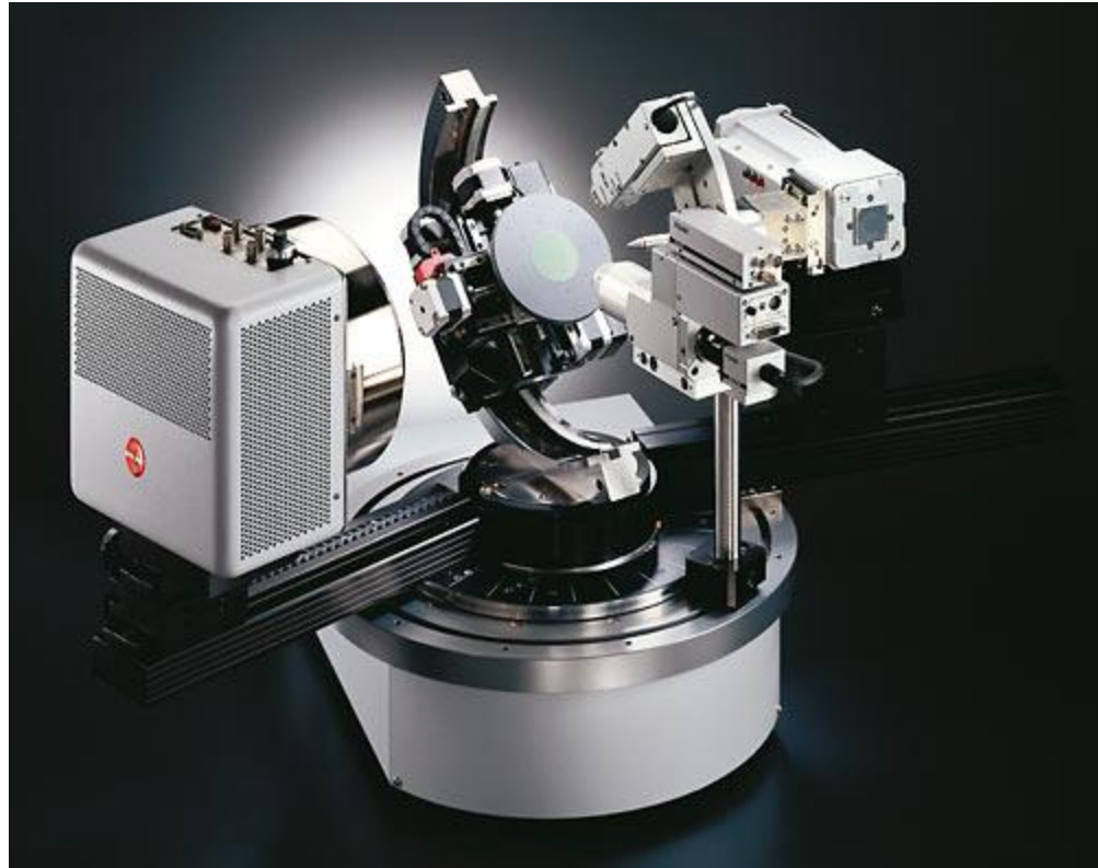
General Area Detector Diffraction System (GADDS)
