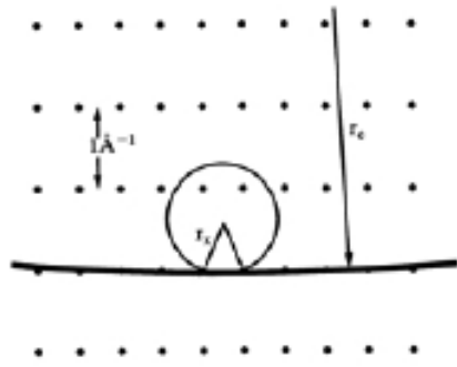
Ewald sphere for Cu radiation is much more curved than that for electrons in an electron diffraction experiment
